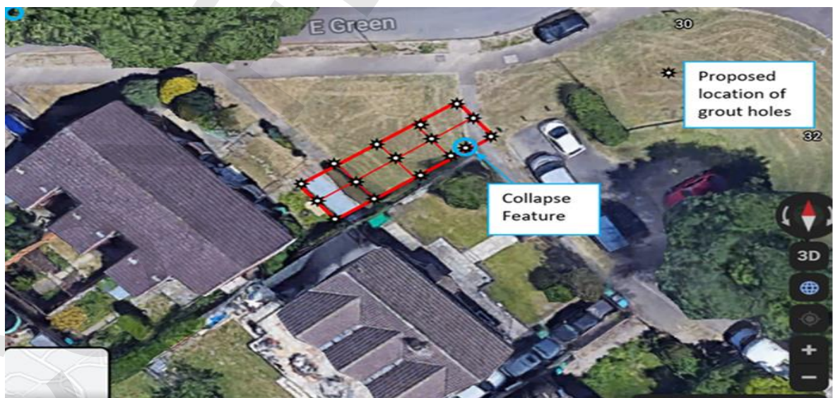
Figure 4 Scope of the identified void
